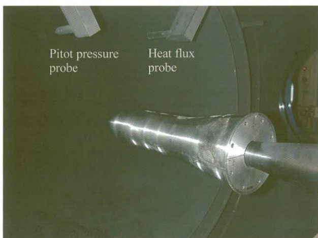
Fig. 5 Heat model installed in the test section.
