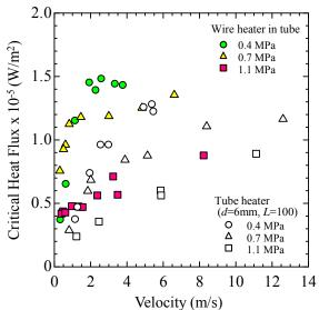
Fig. 3. Effect of flow velocity on critical heat flux.
