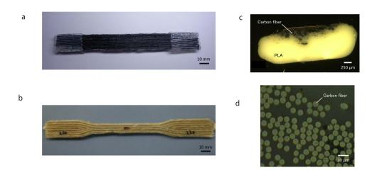
**Figure 2.** 3D-printed (a) CFRTP and (b) dumbbell-shaped JFRTP tensile test specimens. (c) Cross-section and (d) magnified cross-section of the CFRTP specimen.
