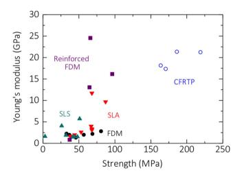
Figure 6. Young's moduli and strengths of continuous carbon-fiber composites fabricated in the present study compared with composites fabricated by FDM<sup>21,23,25</sup> and using commercially available 3D printers, such as SLS<sup>48</sup>, SLA<sup>48</sup>, and FDM<sup>49</sup>.
