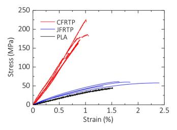
Figure 3. Stress-strain curves of PLA, unidirectional CFRTP, and unidirectional JFRTP specimens fabricated by 3D printing.
