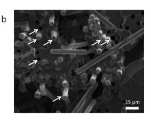
**Figure 5. Fracture of a unidirectional continuous FRTP fabricated by 3D printing.** Fiber pullout due to tensile fracture observed as an **(a)** overview and **(b)** scanning electron microscopy image of the CFRTP specimen. **(c)** Fiber pullout in the JFRTP specimen.
