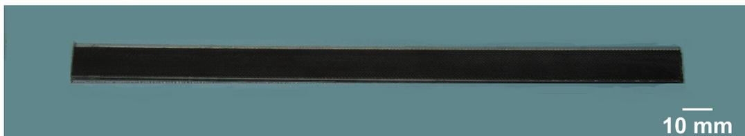
**Figure 5.** Sample with 6 layers of CFRTP printed by the Mark One<sup>®</sup>. The sample still has to be ground and the tabs still have to be at-
