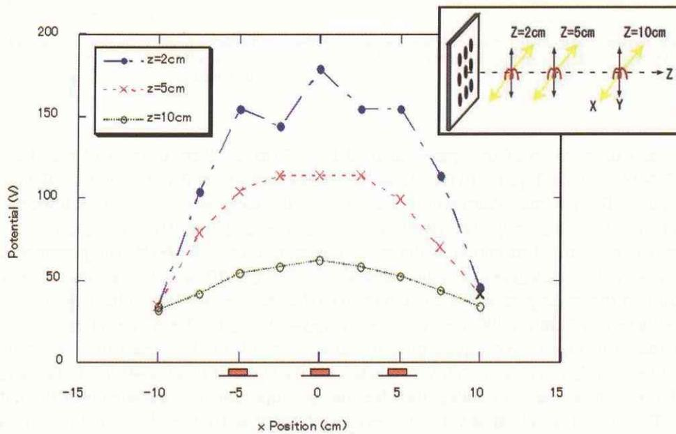
Fig. 13 Distribution of the space potential when the array voltage is 400 V.
