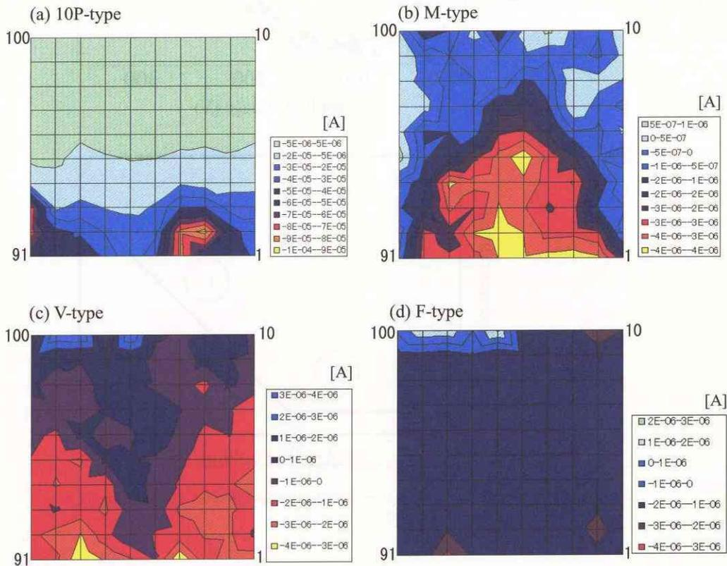
Fig. 7 Distribution of the electrode current. The intersection point on each coordinate is the position of the electrode.
