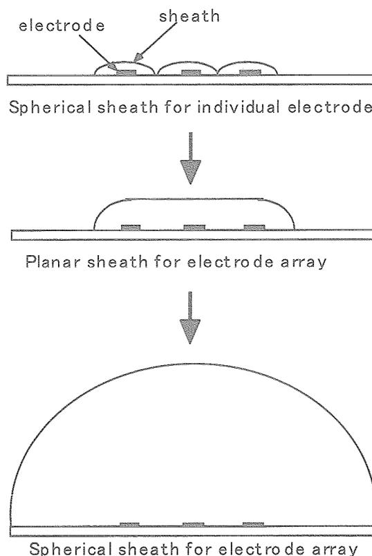
Fig. 16 A model of the growth of the sheath as the bias voltage increases.
