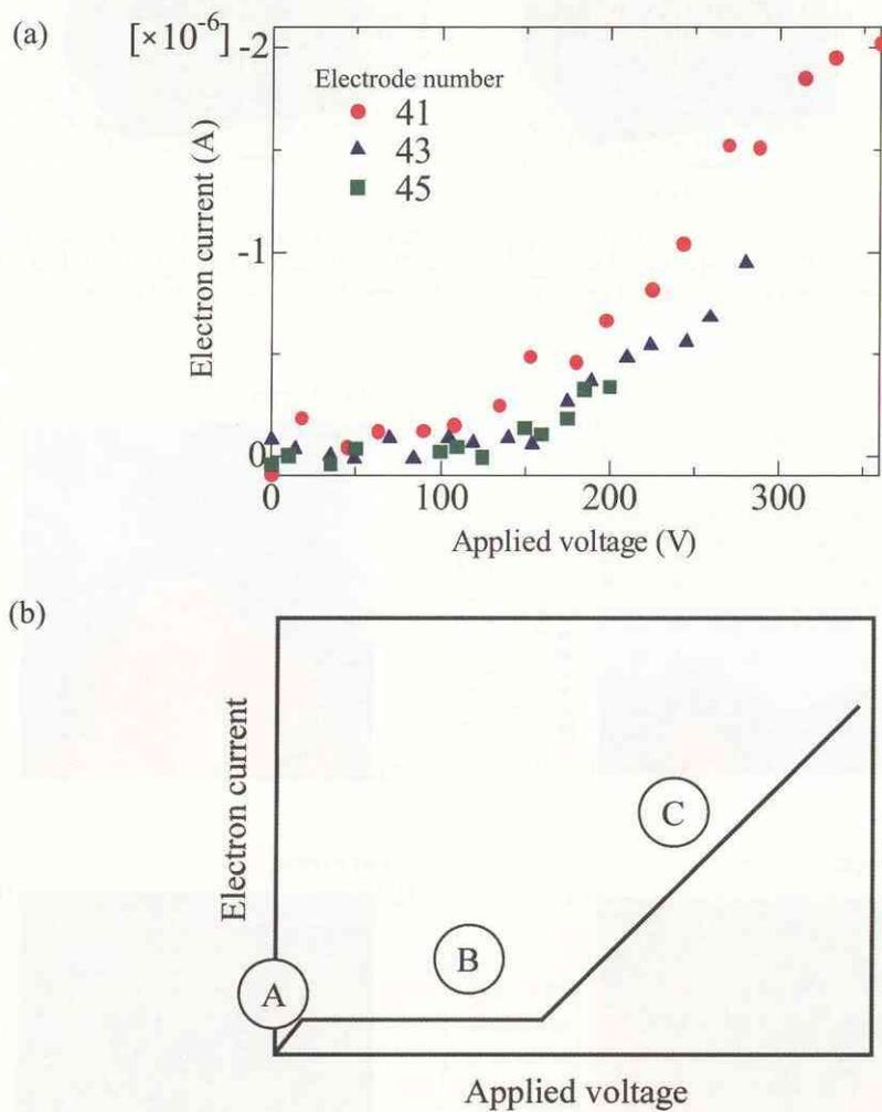
Fig. 9 (a) Electrode current for the voltage distribution for 10P-type. (b) Three stages in the voltage-current characteristics.
