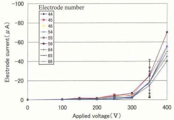
Fig. 11 Voltage-current characteristics when the bias voltage from 0 to 400 V is applied to the electrodes at the same time.
