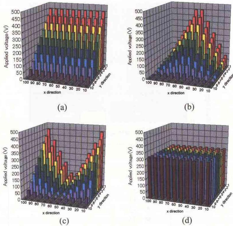
Fig. 6 4 kinds of voltage distribution profile. (a) 10 parallel type. 0-500 V is applied to each line of electrodes. (b) Mountain type. 0-500 V is applied. (c) Valley type. 0-500 V is applied. (d) Flat type. 300 V is applied. Each profile is called in this paper as 10P-type, M-type, V-type and F-type, respectively.
