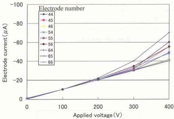
Fig. 10 Voltage-current characteristics when the bias voltage from 0 to 400 V is separately applied to the each electrode.
