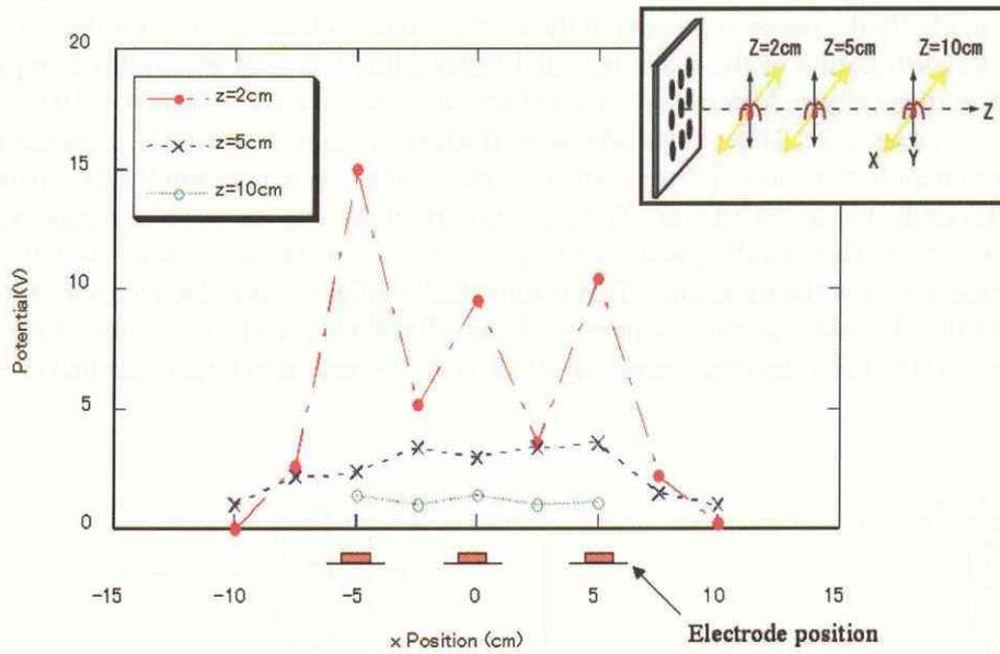
Fig. 12 Distribution of the space potential when the array voltage is 300 V.  $z$  is the distance from the plate and  $x$  is the position parallel to the plate.
