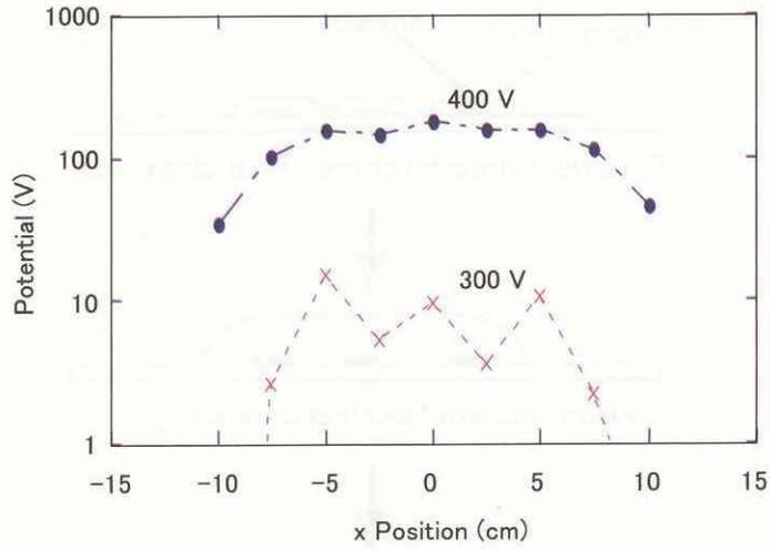
Fig. 14 Distribution of the space potential at 2 cm in front of the array.
