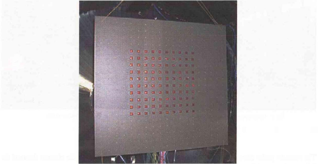
Fig. 4 10 × 10 electrodes on the CFRP panel to simulate the high voltage solar array.
