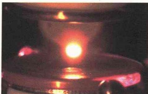
Figure 1 Liquid zirconium at the temperature of 2500 K.
