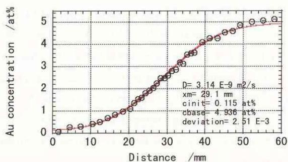
**Fig.3** Concentration profile of Au in Ag melt
