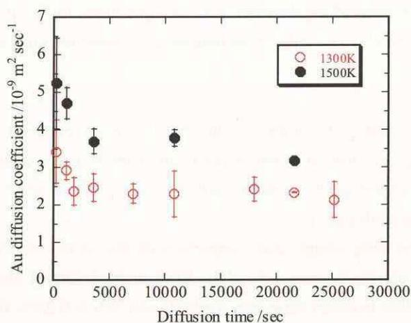
**Fig.4** Time dependence of diffusion coefficient of Au in Ag melt
