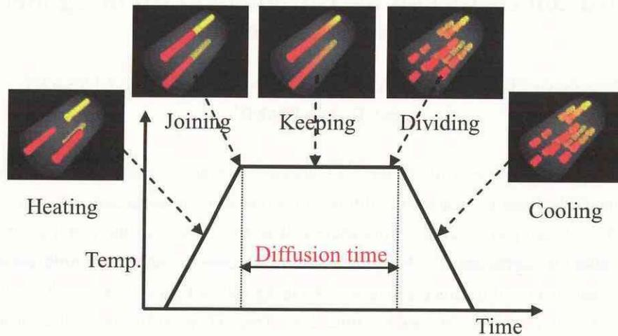
Fig.1 Shear cell method
