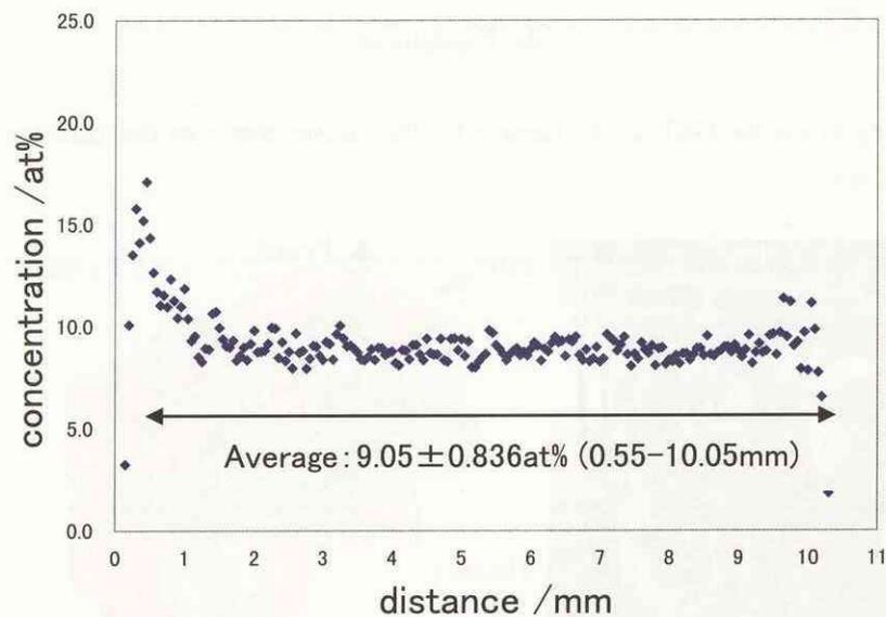
Fig.11 Si concentration in the pellet sample as a function of the distance from the surface along the diameter
