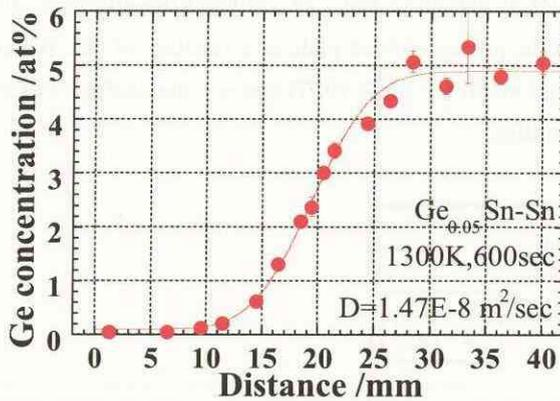
Fig.8 The concentration distribution of Ge in liquid Sn
