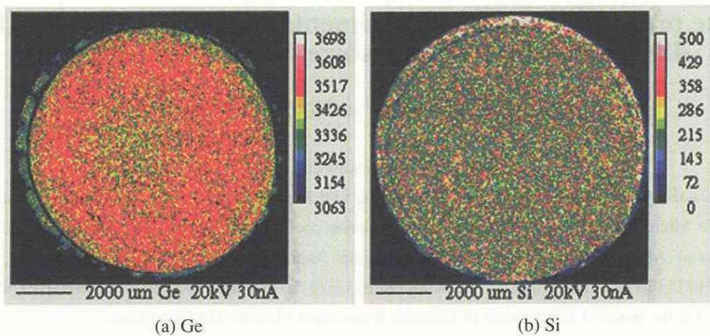
Fig.10 The obtained mapping image of EPMA for Ge and Si
