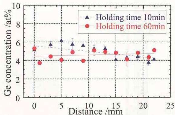
Fig 5 Ge concentration profile before joining the diffusion couple
