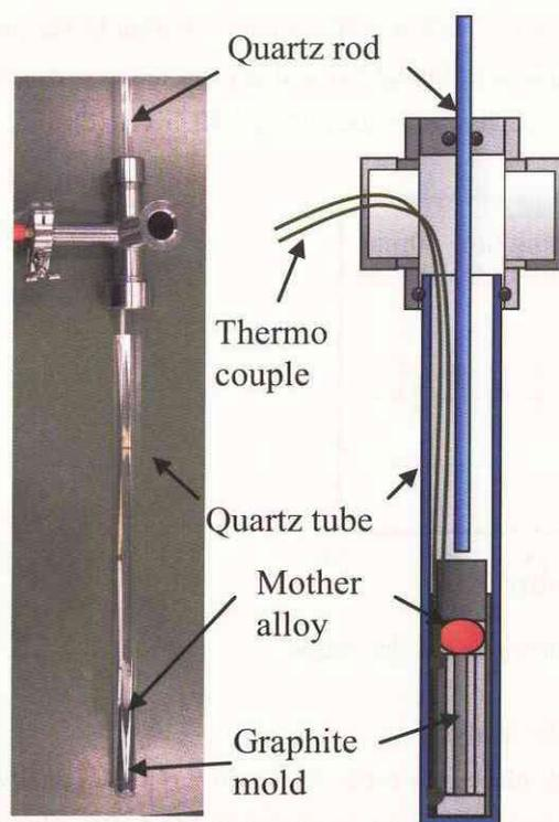
Fig.2 Casting system
