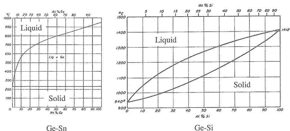
Fig.1 Phase diagram of Ge alloys.
