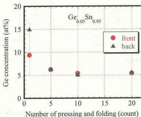
Fig.7 The dependence of Ge concentration on the number of pressing and folding.
