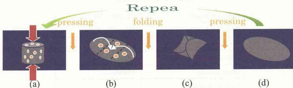
Fig.6 Pressing and folding method for the concentration analysis
