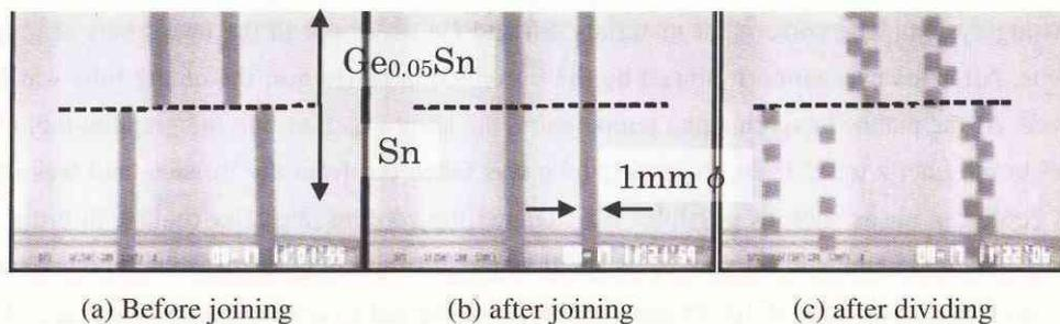
Fig.4 X-ray images of the shear cell operation
