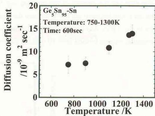
Fig.9 The temperature dependence of the diffusion coefficient
