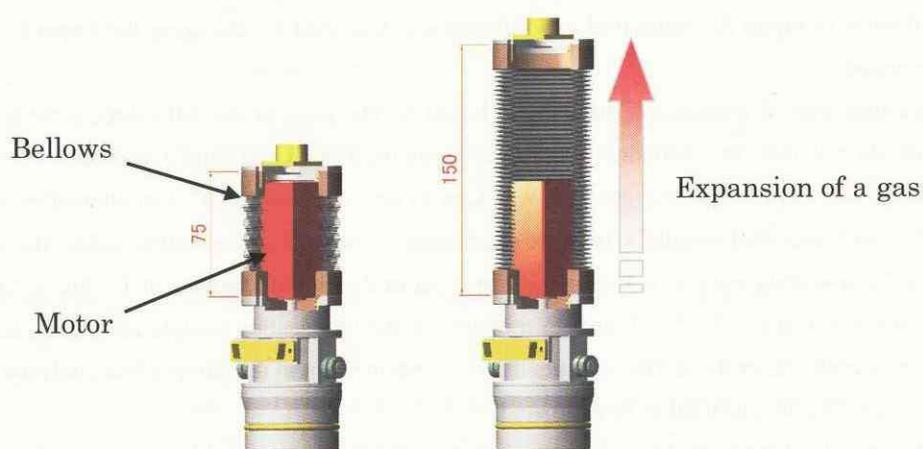
Fig.6 Pressure control and drive part
