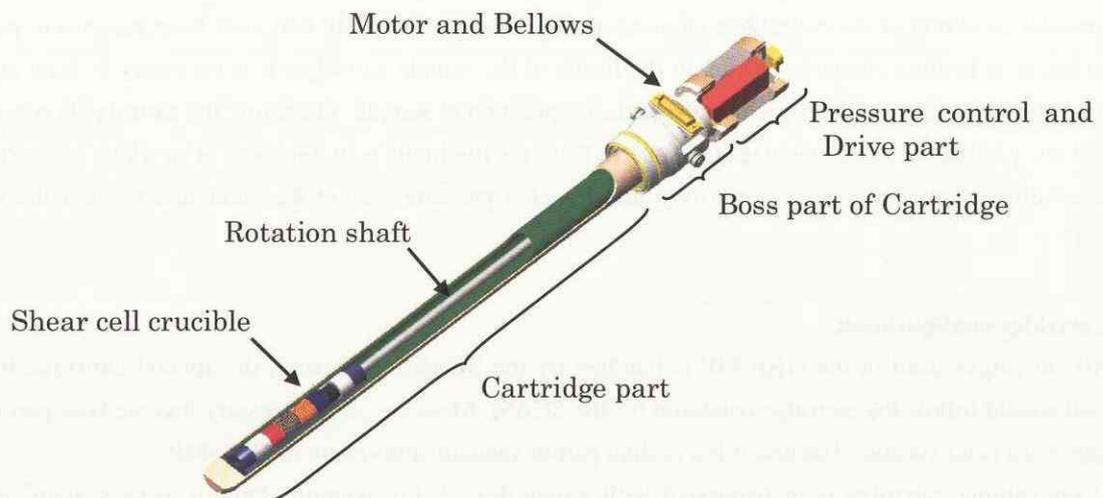
Fig.5 Shear cell cartridge for the GHF-MP
