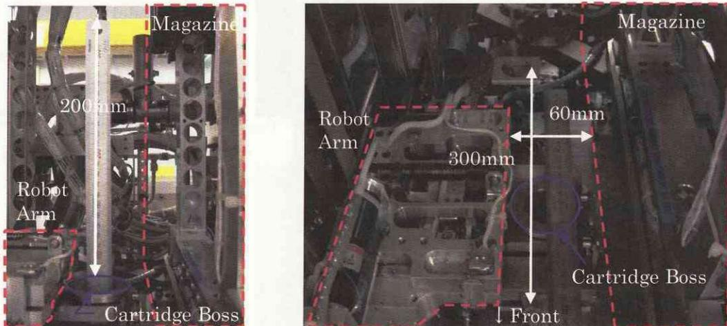
Fig.4 The inside of SCAM
