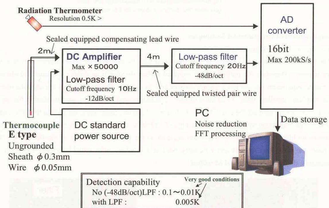
Fig. 2-5 Schematic diagram of temperature measurement system
