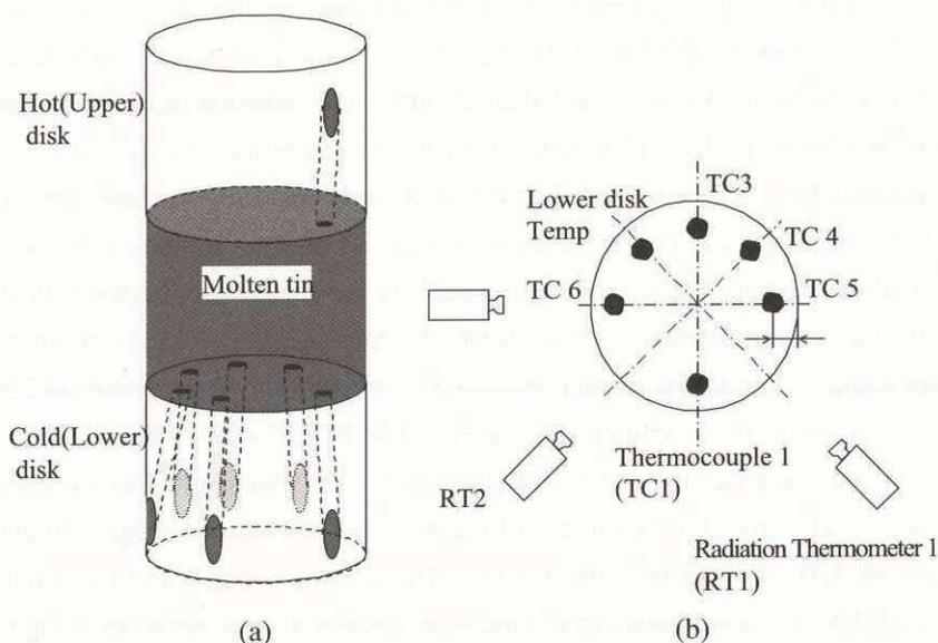
Fig. 2-3 Temperature measurement points
