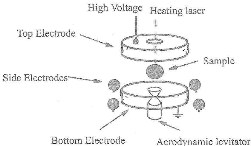
Fig.2. Schematic view of the hybrid electrostatic-aerodynamic levitator
