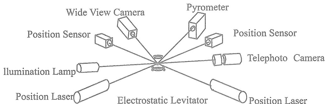
Fig.1. Schematic representation of the facility.
