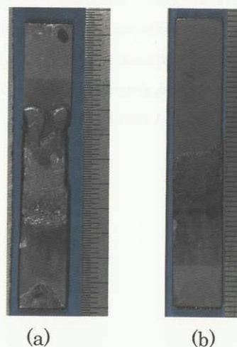
Fig. 9 As grown crystal surfaces without and with boron nitride powder around a seed and a feed: (a) without powder and (b) with powder.
