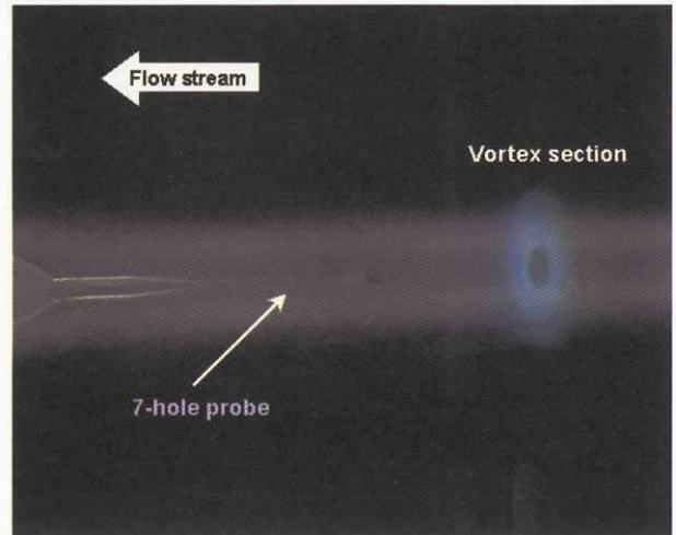
Figure A.6 Tip vortex visualization using LLS (rectangular type tip,  $\alpha=10^\circ$ )
