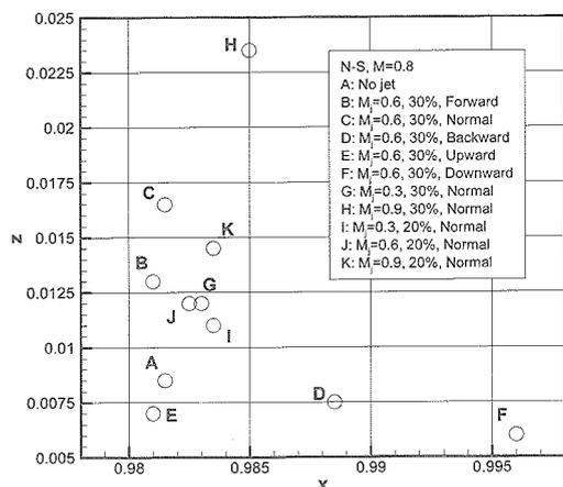
Figure 3.15 Comparison of vortex position in  $x$ - and  $z$ -axis with various jet directions (Navier-Stokes,  $M=0.8$ )
