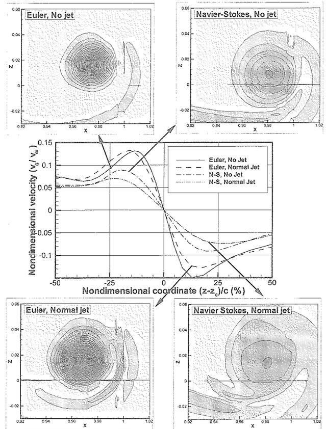
Figure 3.13 Comparison of tip vortex between results of Euler and Navier-Stokes calculations ( $M=0.8, M_j=0.6$ )
