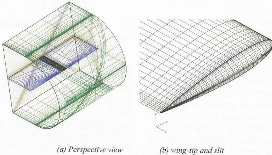
Figure 2.1 H-C-type grid system
