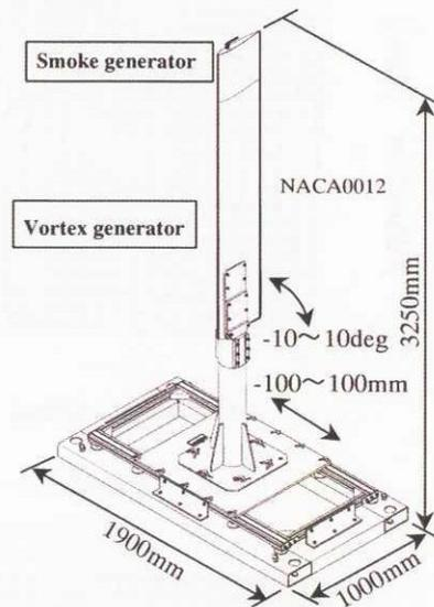
Figure A.3 Diagram of vortex/smoke generator
