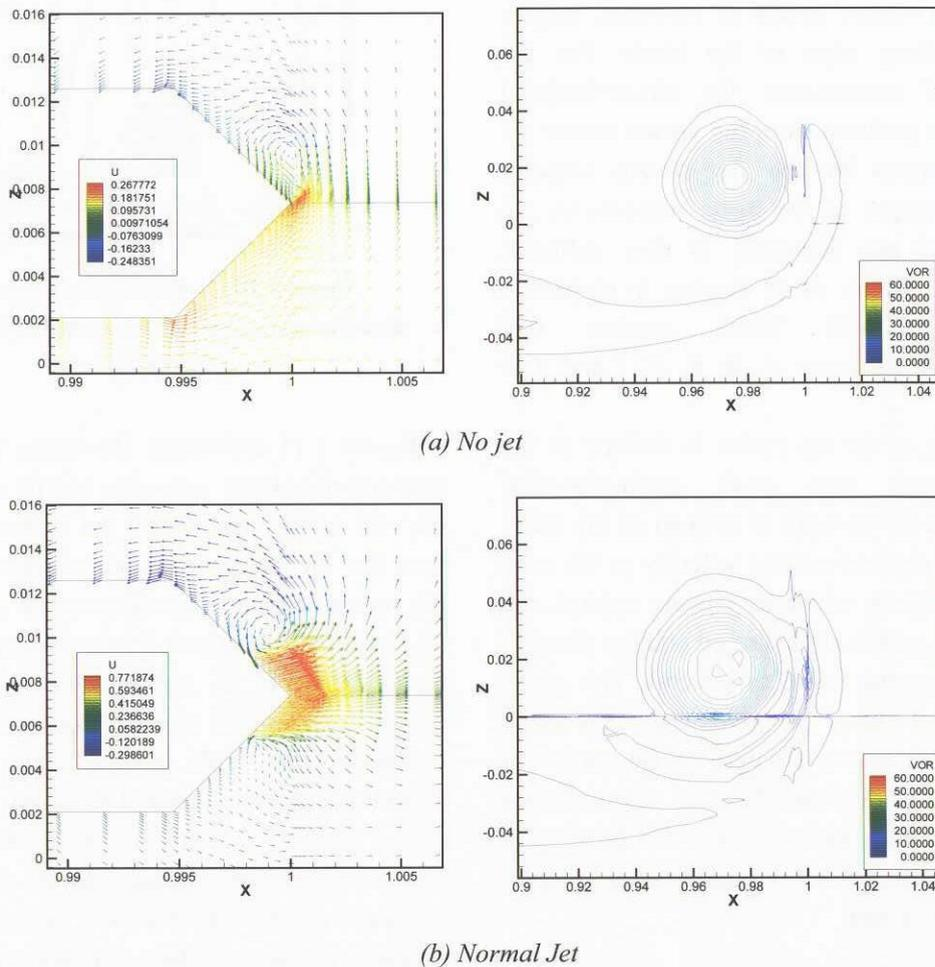
Figure 3.8 Comparison of velocity vectors and contours various jet, directions (Euler  $M=0.8$ ,  $M_t=0.6$ )
