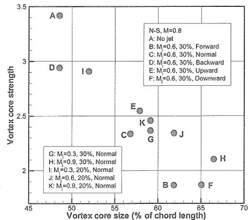
Figure 3.14 Comparison of vortex core size and strength with various jet directions (Navier-Stokes,  $M=0.8$ )
