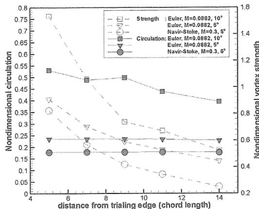
Figure 3.4 Nondimensional circulation at distance from trailing edge for various computations
