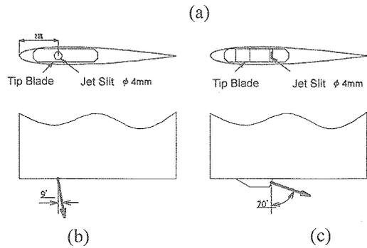
Figure B.4. Jet slit and diagram of jet blowing system with two injection angles
