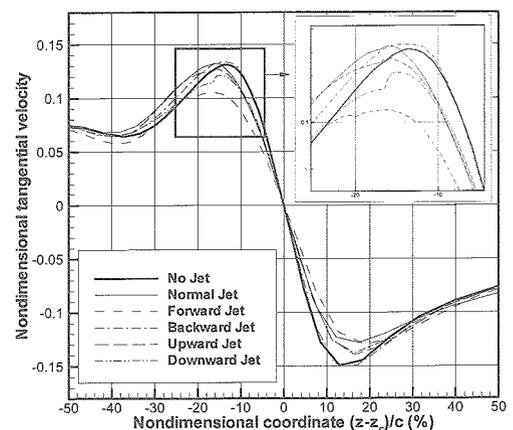
Figure 3.10 Comparison of tangential velocity distributions at  $L=10C$  according to jet directions ( $M=0.8$ ,  $M_j=0.6$ )
