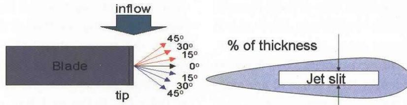
Figure 3.5 Diagram of cases with various tip jet conditions
