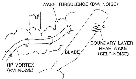
Figure 1.2 Diagram of noise sources in helicopter rotor
