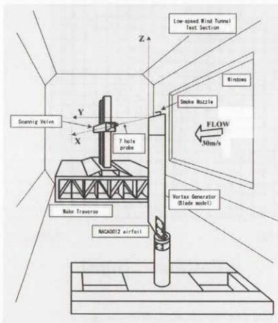
Figure A.1. Diagram of test section equipment system
