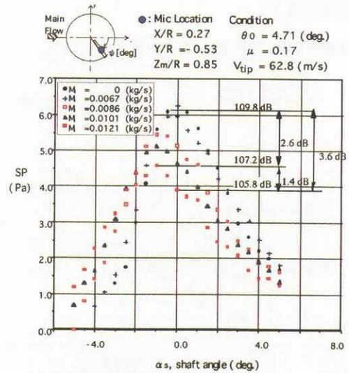
Figure B.6. Comparison of BVI peak of rotor according to tip jet speed ( $V_{tip}=62.8\text{m/s}$ )
