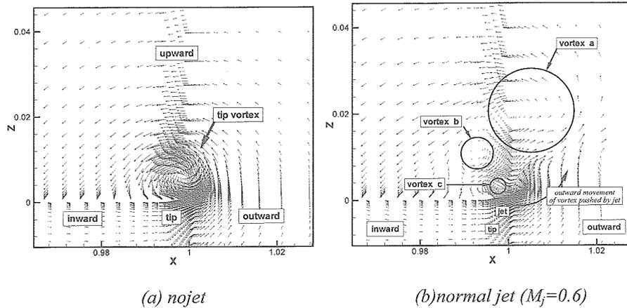
Figure 3.9 Crossflow velocity vectors at mid-section of 90% chord length for tip vortex formation (Euler,  $\alpha = 5^\circ$ ,  $M=0.8$ )
