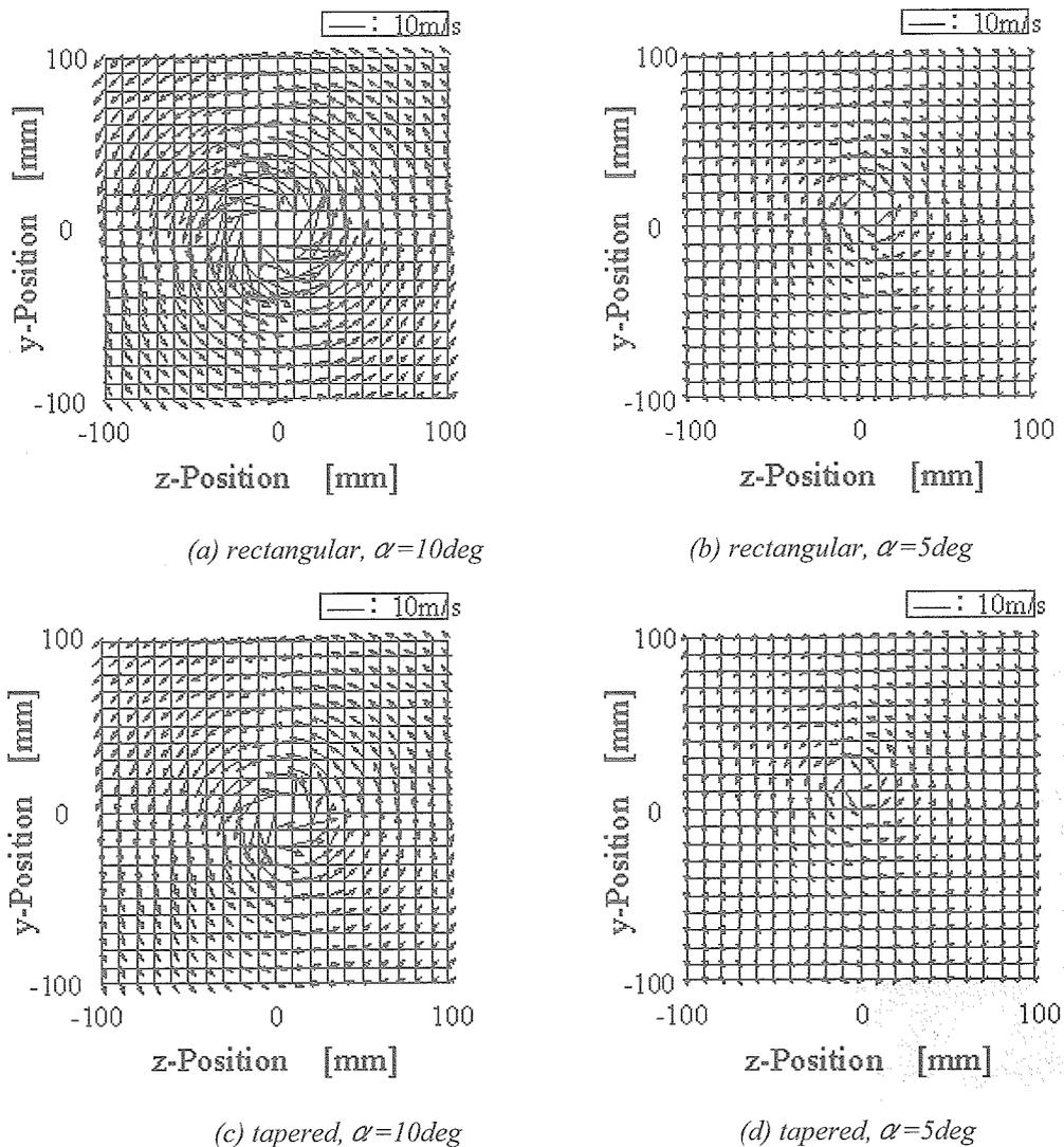
Figure A.4 Vector plot for vertical velocity components,  $v$  and  $w$  (square and tapered, 10mm pitch,  $x/c=14$ )
