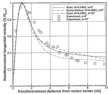
(a) diagram of jet flow near tip (b) Comparison of circumferential velocity profile
