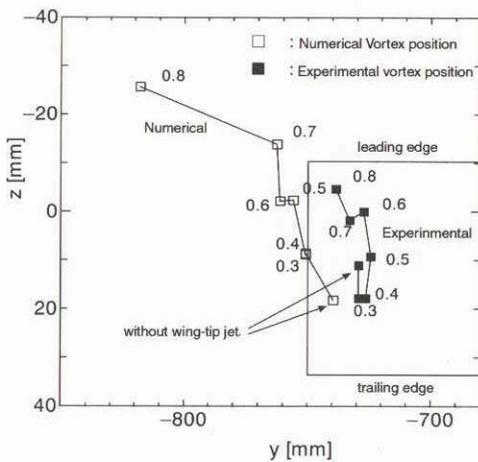
Figure B.5. Comparison of vortex position according to internal pressure for tip jet blowing
