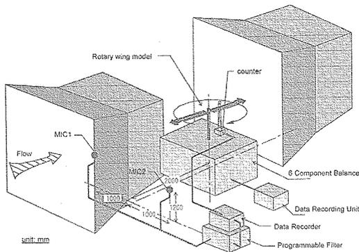
Figure B.2 System diagram of wing-tip blowing experiment with rotary wing
