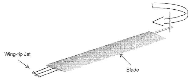
Figure 1.4 Diagram of wing-tip blowing jet of rotor
