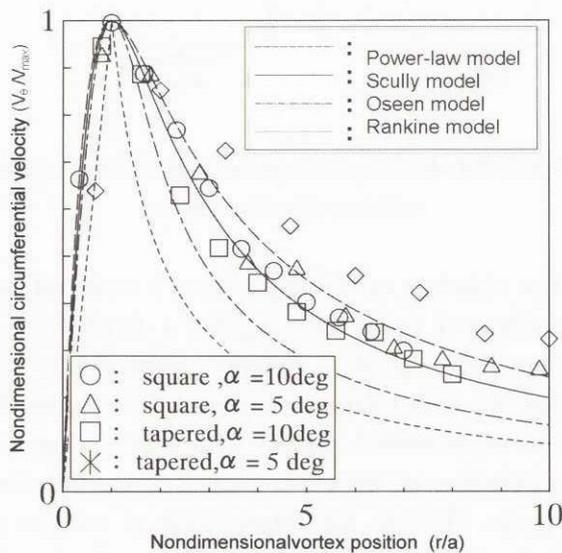
Figure A.5 Comparison of circumferential velocity profiles of tip vortices (rectangular;  $\alpha=10\text{deg}$ ,  $x/c=5$ )
