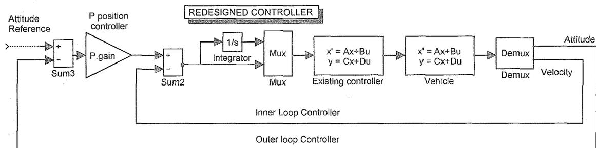
Fig. 2. Redesigned cascade controller.
