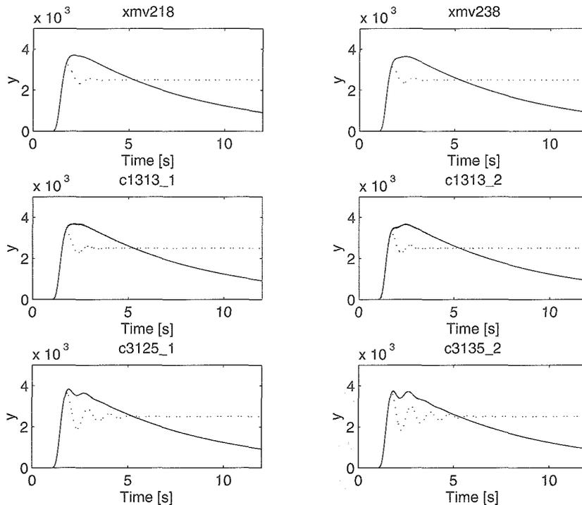
Fig. 7. Time domain responses to an input step disturbance (controller e9\_8a\_3).
