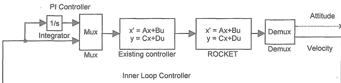
Fig. 1. Inner loop (attitude angular velocity) controller, having an integral compensation.
