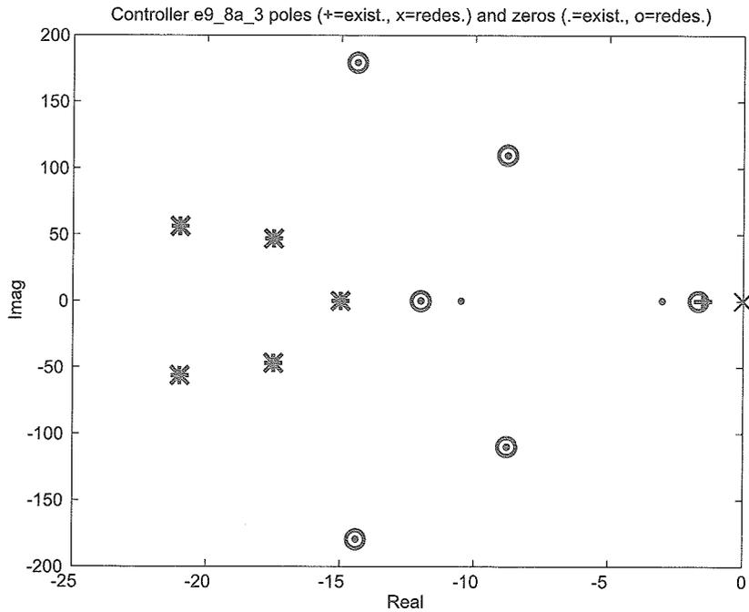
Fig. 5. Zero-pole map of the existing (e9\_8a\_3) controller and its redesigned version.
