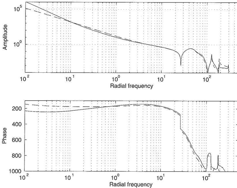
Fig. 6. Bode plots of the e9\_8a\_3 controller and its redesigned version.
