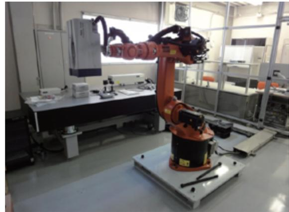
Fig.1.2 Compact Multi-axial Vibration Evaluating System (MaVES-c)
