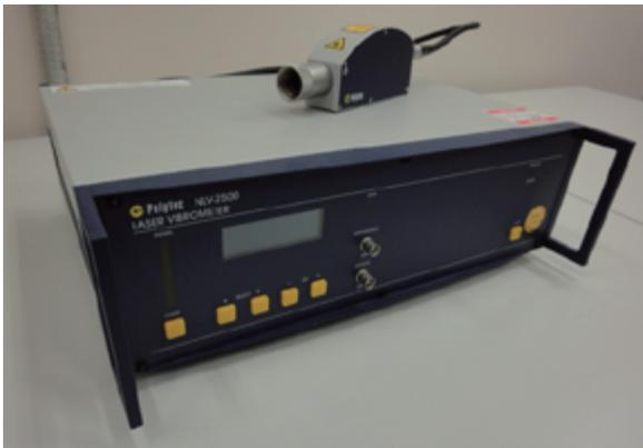
Fig.3.18 Laser vibrometer (NLV-2500)
