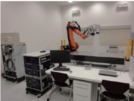
Fig.1.1 Multi-axial Vibration Evaluating System (MaVES)
