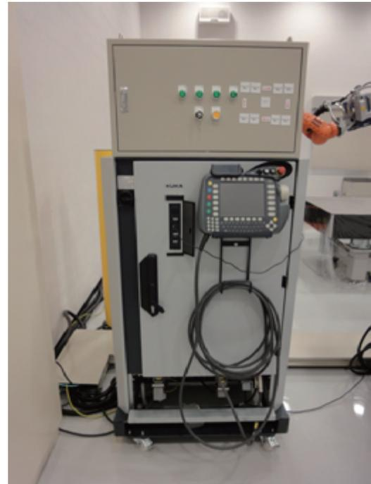
Fig.3.7 Robot control device and teach pendant KCP
