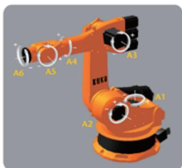
Fig.3.10 Axes of robot
