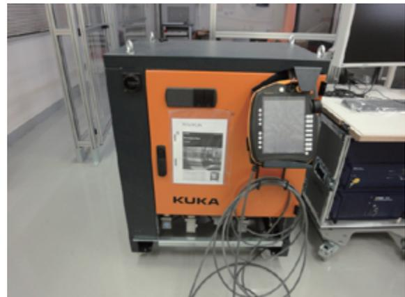
Fig.4.5 Robot control device and smartPAD
