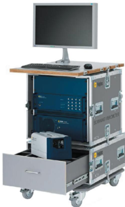
Fig.4.2 Configuration of 1D scanning vibrometer (rack)
