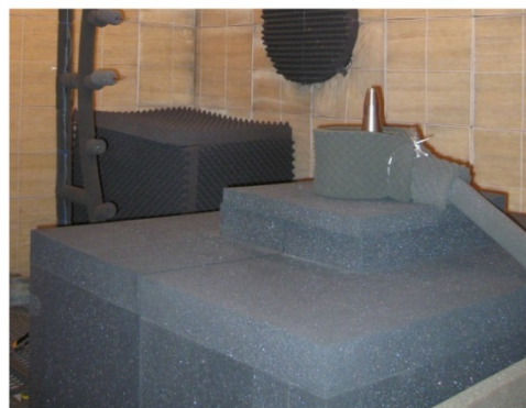
Fig. 8 Settling chamber, covered by acoustic absorption material.
