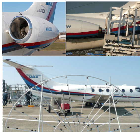
Fig. 4 Engine test using a low-bypass-ratio turbofan engine installed on jet plane. Top left : the tested engine (JT15D), top right : a pressure rake and the traversing system placed behind the engine. Bottom : a simple phased array microphone to detect noise sources around the engine.
