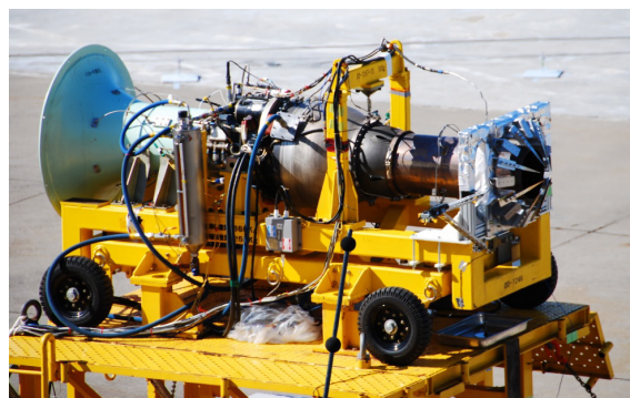
Fig. 3 Demonstrator engine in an outdoor test configuration. A claw mixer is placed at the nozzle (FY2011 version).
