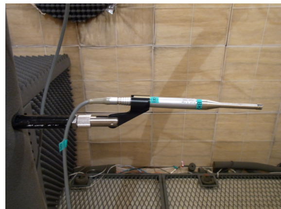
Fig. 10 Microphone cartridge, adapter, preamplifier, microphone holder, and microphone cable.
