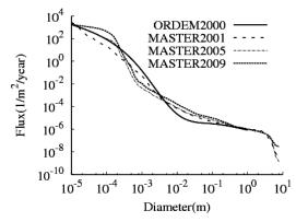
Figure 4. Debris impact flux against the debris diameter for GCOM-W1 as calculated for each model's threshold year.
