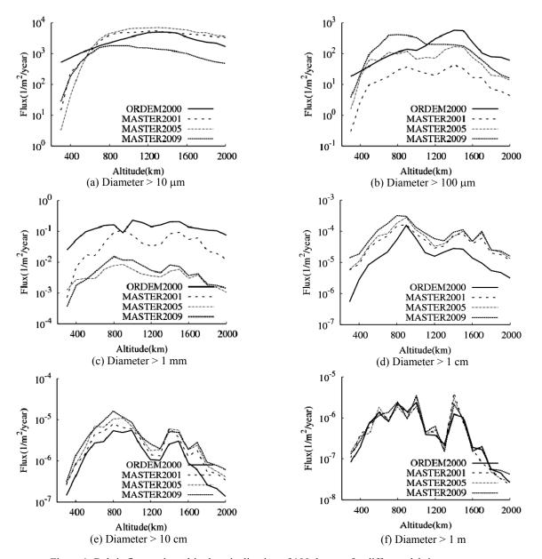
Figure 1. Debris flux against altitude at inclination of 100 degrees for different debris
