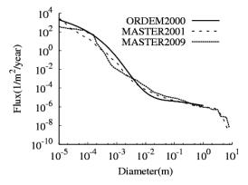
Figure 5. Debris impact flux against the debris diameter for GCOM-W1 as calculated with each model for the year 2012.
