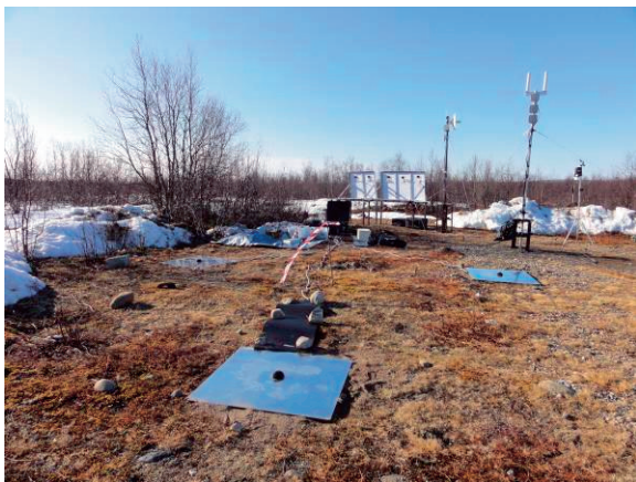
Fig. 2-3 Ground microphone setup
