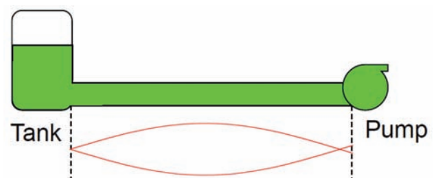
Fig. 3 Mode shape of pressure oscillation in a feed line
