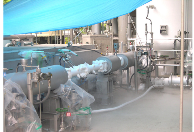
Figure 2 Overview of the Cryogenic Cavitation Tunnel (CCT)
