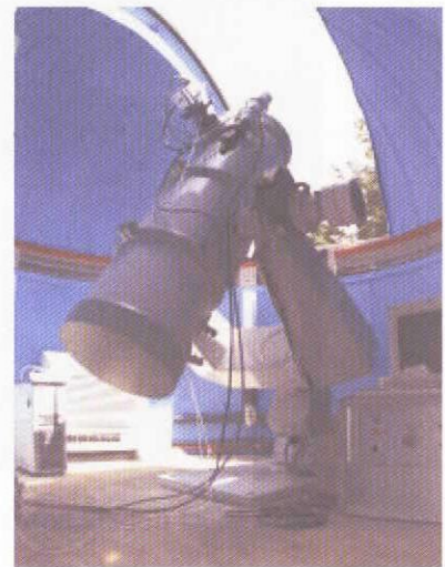
Fig.3 Equatorial-mount 35cm telescope at Nyukasa-yama
