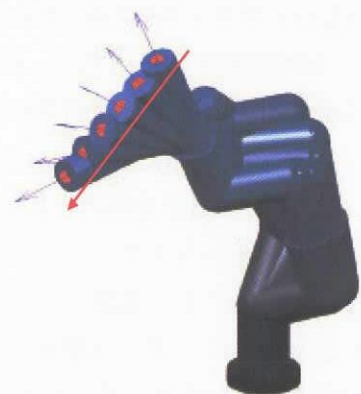
Fig.3 Interplated linear motion by solving inverse kinematics
