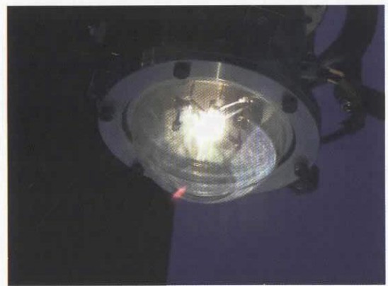
Fig. 4 Thruster in solar heating
