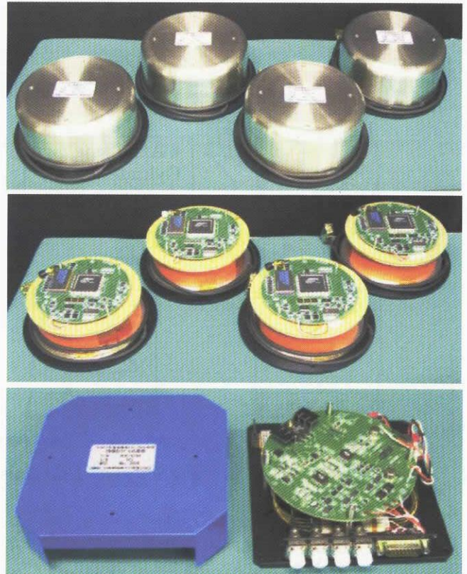
Fig.5 : 2 nd Experimental Model(EM 検討モデル) Upper : Coil (4 sets) Middle : Coil (Inner Side) (4 Sets) Lower : Light Source (1 set for 4 Coils)
