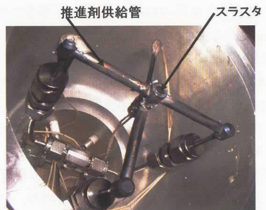
Fig. 2 Standard type thruster
