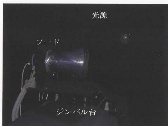
Figure 5 Experimental Configuration of Stray Light
