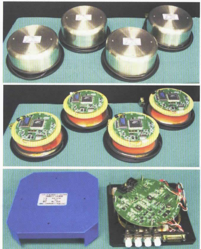
Fig.5 : 2 nd Experimental Model(EM 検討モデル) Upper : Coil (4 sets) Middle : Coil (Inner Side) (4 Sets) Lower : Light Source (1 set for 4 Coils) RIN比較 (IF=200mA)
