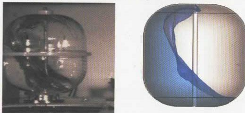
Fig.3-2-3 Sloshing in the Model Tank without Anti-slosh Devices; Experiment and Computation (t=0.48sec)
