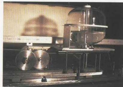
Fig.3-2-2 Model Tank Mounted on the Mechanical Exciter
