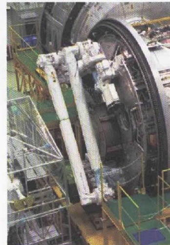
Fig. 2.2-10 JEMRMS flight model
