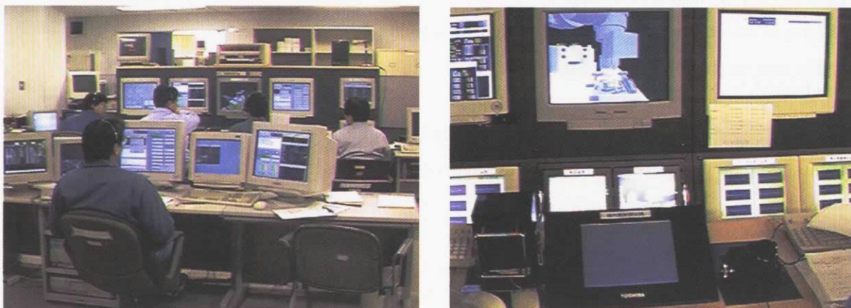
Fig.5.1.9.2-1 ETS-VII's teleoperation system
