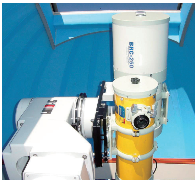
Telescope: Takahashi BRC-250 D: 250mm f : 1268mm (F/5.1) Equatorial mount: Showa eccentric elbow-type 25EL
