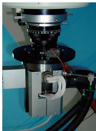
CCD camera: N.I.L. CCD44-82x2 chip: 2K4K back-illuminated (e2v) × 2 cooling: circling refrigerant(-100°C) FOV: 2.78 × 2.78°
