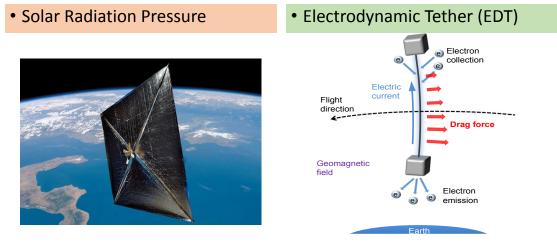
✓ Solar – simple, slow; deal with stability, durability, & collision cross-section issues
