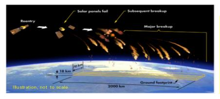
Micro satellites and smaller satellites will pose little air or ground impact risks - Beware of densely-built components such as control moment gyros and batteries
