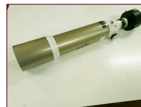
FASTSCOPE: 10 cm diameter telescope The total field of view is about 0.5^\circ \times 0.5^\circ
