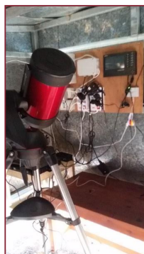
EQUO OS: 15.0 cm diameter. The total field of view is about 0.5^\circ \times 0.5^\circ degrees
