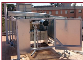
MITO: 25.0 cm diameter. Total field of view is about 3.5^\circ \times 2.5^\circ
