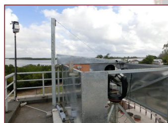
EQUO OG: 25.0 cm diameter telescope The total field of view is about 2.2^\circ \times 2.2^\circ
