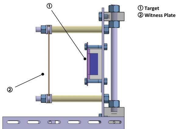
Figure C.1 — Sketch of target and witness plate assembly
