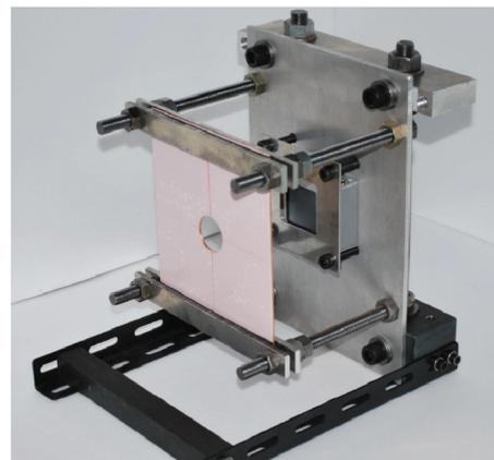
Figure C.2 — Picture of target and witness plate set-up
