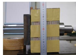
Fig. Sampler fixed in impact axis.
