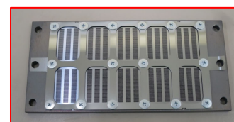
Field Emission Cathode for KITE
