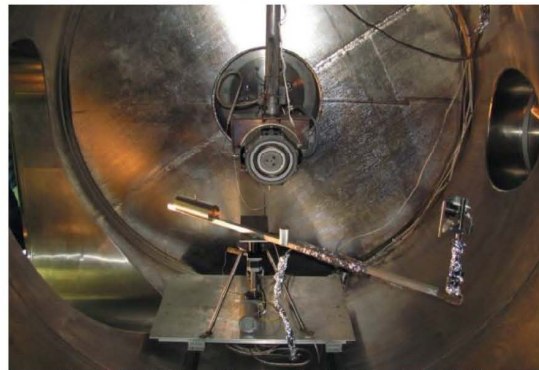
Figure 4. PlaS-120CM ser.01 in vacuum chamber of the Y-2B-2 test facility with the probe movement device
