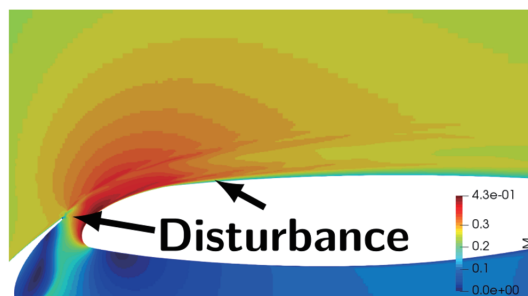
Total C_l and M Distribution for \alpha = 5.5 deg, Level 5 Adapted Grid
