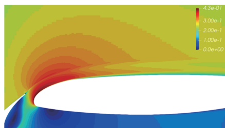
Total C_l and M Distribution for \alpha = 5.5 deg, Level 5 Adapted Grid
