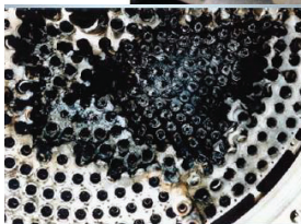
SSME injector damage
