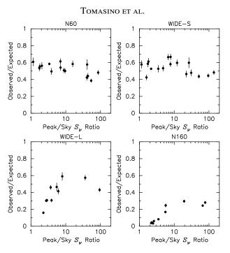
**Figure 1.** The Observed over Expected flux ratio vs. the Peak/Sky surface brightness ratio shows the effect of the slow transient response from a contour aperture by using a contour aperture to account for extended emission.
