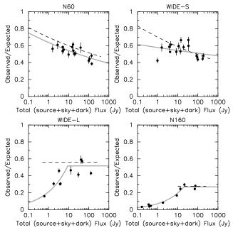
**Figure 2.** The Observed over Expected flux ratio vs. the Total (Observed plus sky and dark) flux plot. The dashed lines represent the fit determined from Shirahata et al. (2009) and the gray is the fit for extended emission.
