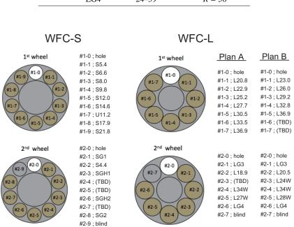
Figure 1. Available slots for filters and grisms for WFC-S and WFC-L.
