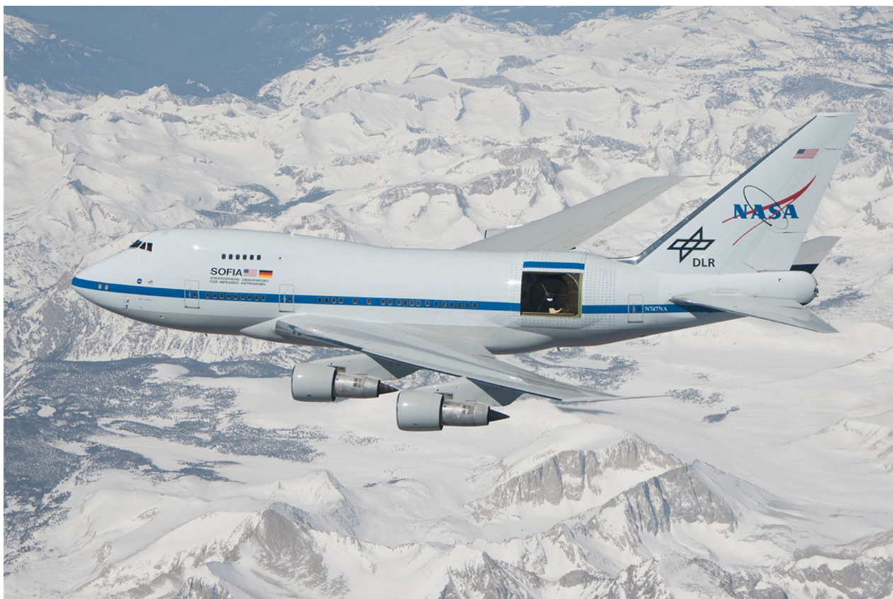
Figure 1. An unusual picture of the SOFIA observatory in flight with the telescope door open in the daytime. The SOFIA observatory does not generally fly with the door open while the sun is up in order to mitigate the risk of focused sunlight inside the telescope cavity. When this picture was taken the telescope's primary mirror was covered with a protective tarp that was developed for open-door aircraft flight testing.
