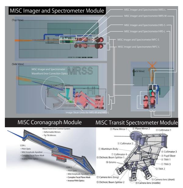
Figure 2. The 3D sold model of the MISC I& S module, MISC COR module and MISC TRA module.
