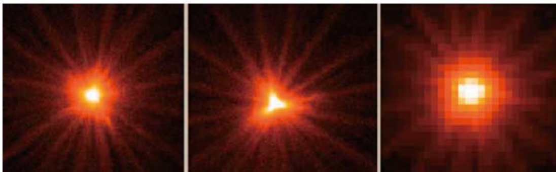
Figure 3.13: On-axis images of the MOS-1 ( left ), MOS-2 ( center ), and pn ( right ) X-ray telescopes ( XMM-Newton Users Handbook 2010 [188] ). These images are 110'' in width, and a square root intensity scale has been used to visualize the wings of the PSF.
