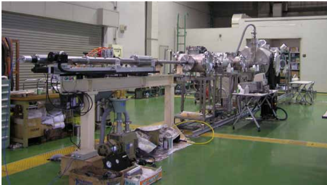
Fig. 2. Two-stage light gas gun and experimental chamber.
