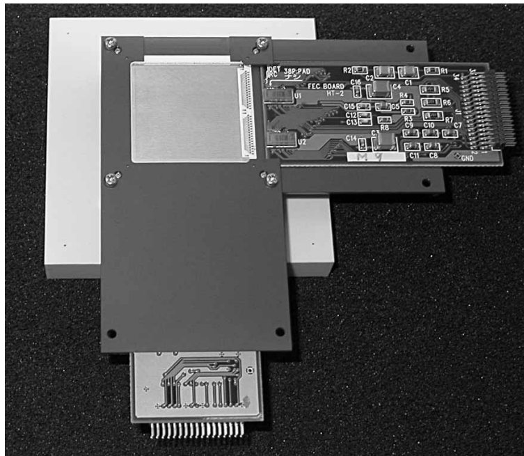
Figure 8.12 Photo of a double-sided CdTe strip detector. The effective area of the detector is 2.56 \text{ cm} \times 2.56 \text{ cm} , and the strip pitch is 400 \mu\text{m} .
