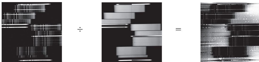
Figure 4.9: Example of a dark subtracted frame (left), a flat frame (middle), and flat-fielded frame (right) of mask R1 chip2.
