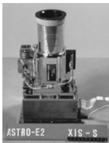
Figure 3.8 A photograph of one of the XIS sensor.
