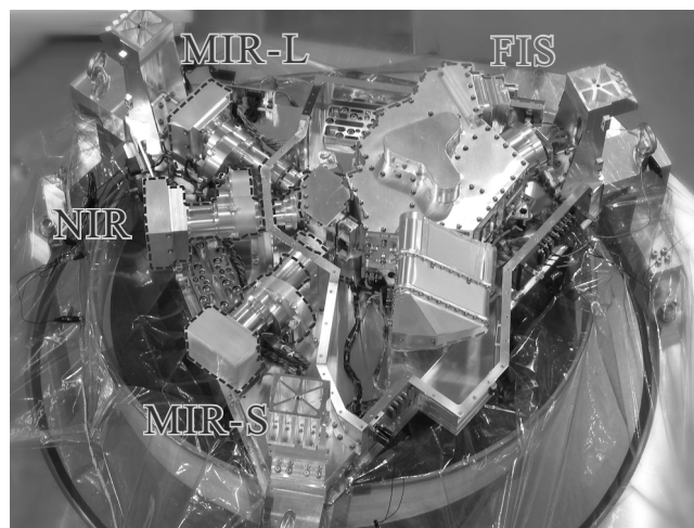
Figure 2.4 Picture of the the Focal-Plane Instruments on board AKARI, located at the backside of the prime mirror.
