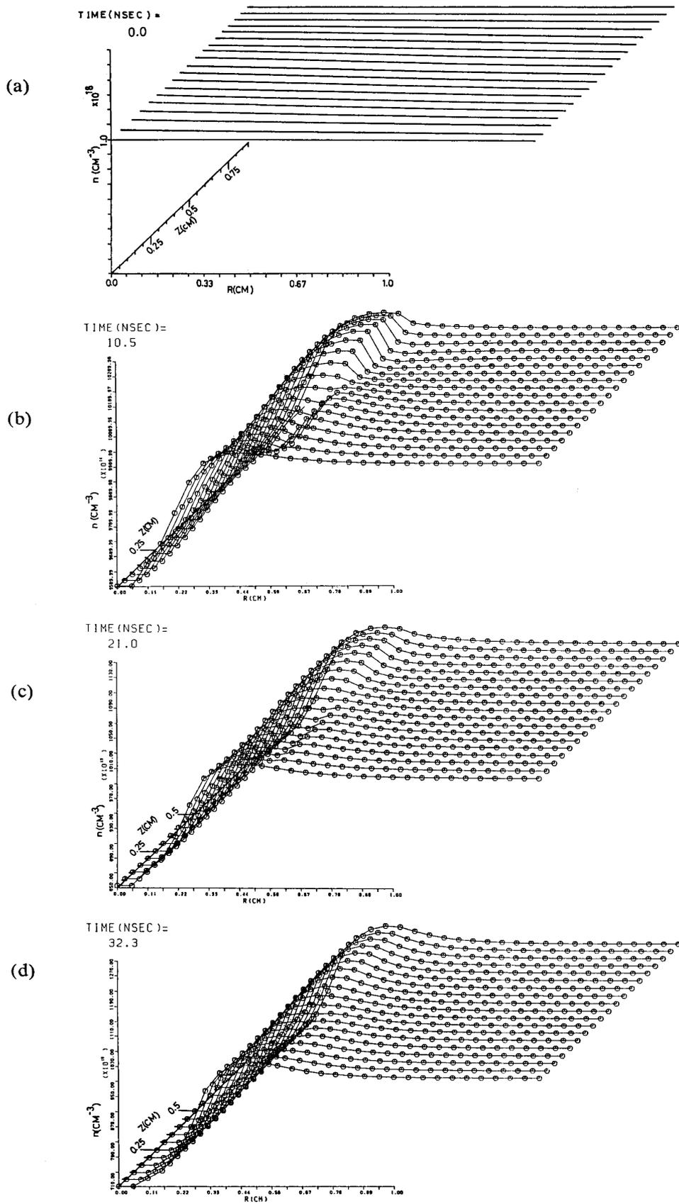
Fig. 1. (a~d) The time sequences of the number density for the argon channel plasma. The radial expansion slightly occurs but is not severe. The sausage instability does not grow so heavily.
