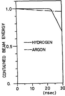
Fig. 5. The diagram for the contained beam energies within the channel radius of 0.5 cm versus the time. The contained energy is normalized by the initially contained one within the channel radius. In the case of the argon channel, the contained energy decreases only by the collisional loss. On the other hand, in the case of the hydrogen plasma channel, the contained energy decreases much mainly by the radial expansion.
