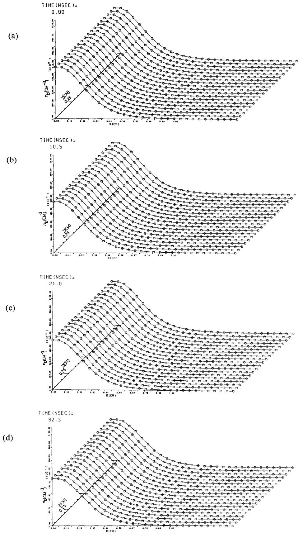
Fig. 3. (a~d) The time sequences of the temperature for the argon channel plasma.
