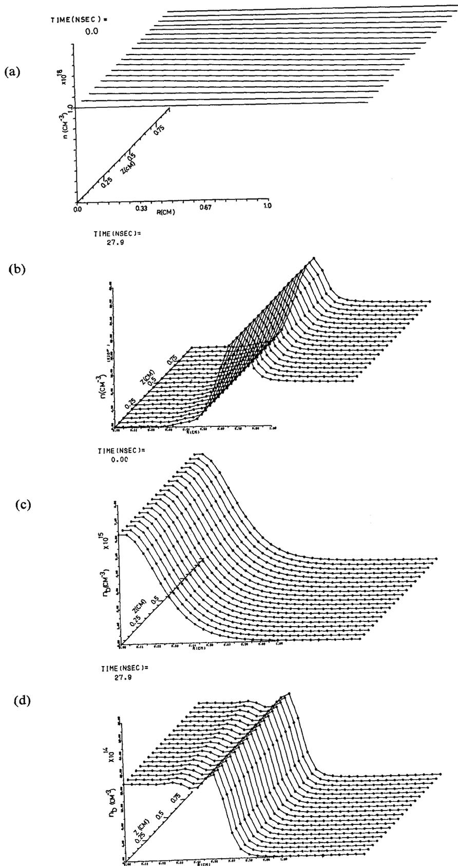
Fig. 4. (a~d) The time sequences of the number density ((a) and (b)) and the beam number density ((c) and (d)) through the hydrogen plasma channel.
