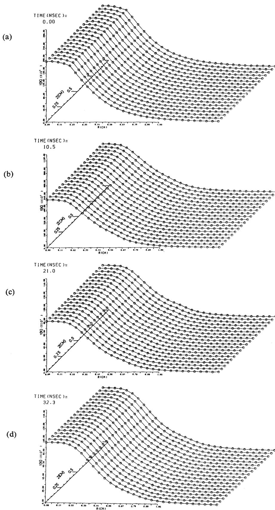
Fig. 2. (a~d) The time sequences of the temperature for the argon channel plasma.
