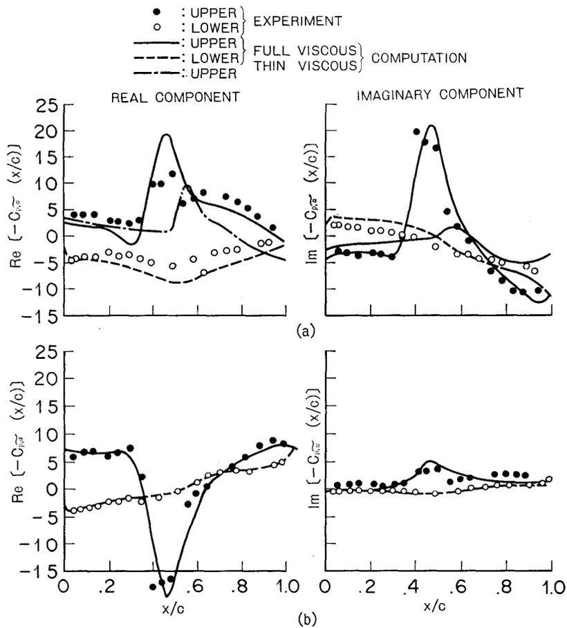
Fig. 5. Response Characteristics of the Airfoil Surface Pressure (Fundamental Mode).
