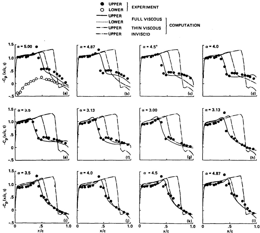
Fig. 3. Instantaneous surface Pressure Distributions ( $K=0.2$ ).
