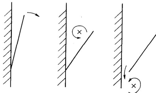
Fig. 4. Two-dimensional Weis-Fogh lift generation mechanism. Only the half portion of the symmetrical configuration is shown.
