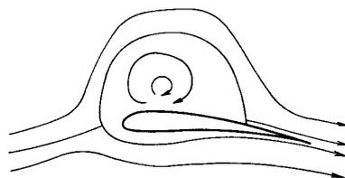
Fig. 3. Schematic flow pattern around an airfoil with a vortex trapped on the upper surface.
