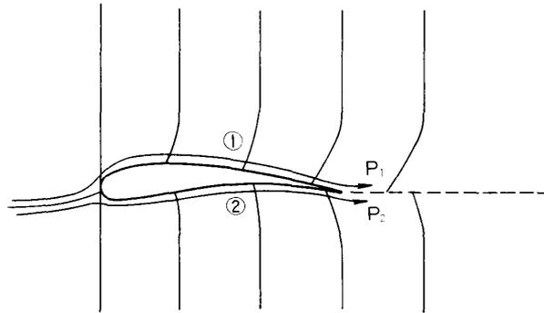
Fig. 1. Particle traces placed originally along the vertical line at the leading edge. Each line shows successive trace after impulsive start.
