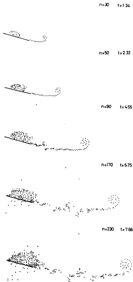
Fig. 2. Discrete vortex simulation of the flow around an impulsively started flat plate at successive time instants.
