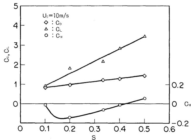
Fig. 8. Aerodynamic forces predicted by numerical simulation.  $C_D$ ,  $C_L$  and  $C_M$  correspond to the lift, drag and moment coefficients, respectively.  $S$  is the Strouhal number of the rotation which was assumed to be constant.
