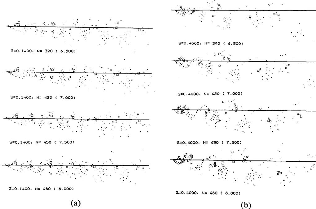
Fig. 7. Numerically simulated vortex distributions along the wake with the Strouhal numbers of 0.14 as (a) and 0.4 as (b). The patterns correspond to each half cycle of rotation.
