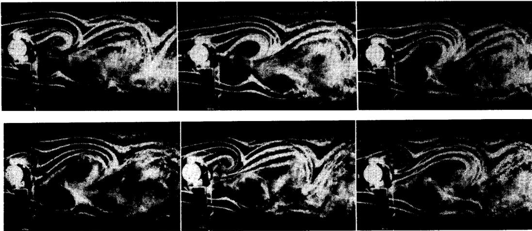
Fig. 5. Flow fields around an autorotating elliptic airfoil visualized by smoke wire method. The field was illuminated by multi-flashed strobo-light synchronized with the autorotation phase. The pictures were taken at each 30 degree phase angle.
