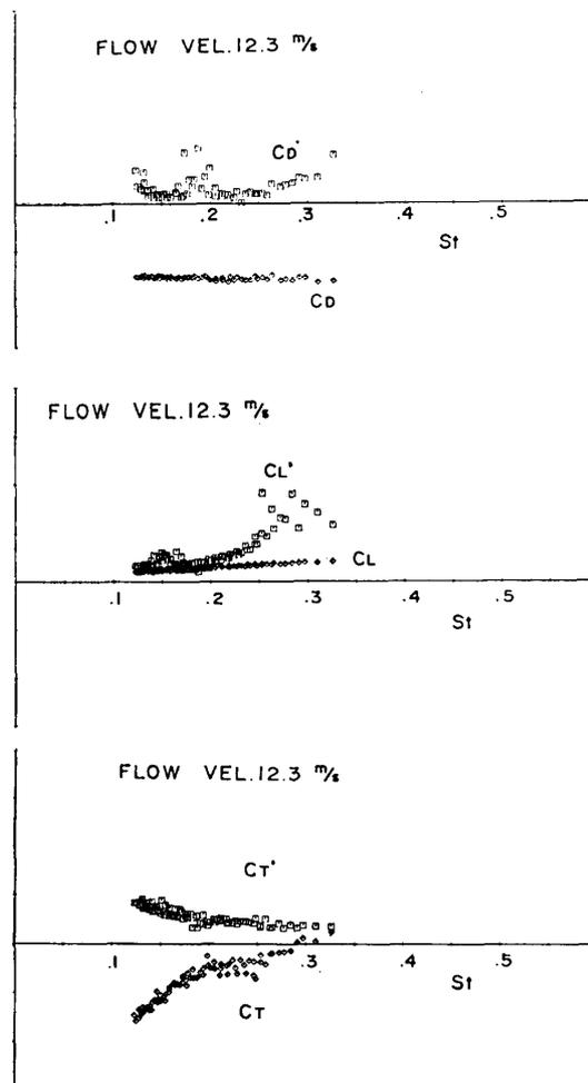
Fig. 9. Aerodynamic forces measured by wind tunnel experiment.  $C_D$ ,  $C_L$  and  $C_T$  correspond to the drag, lift and torque coefficients, respectively, and the primes denote the root mean square deviation over one cycle of rotation.  $St$  is the Strouhal numbers of the forced rotation.
