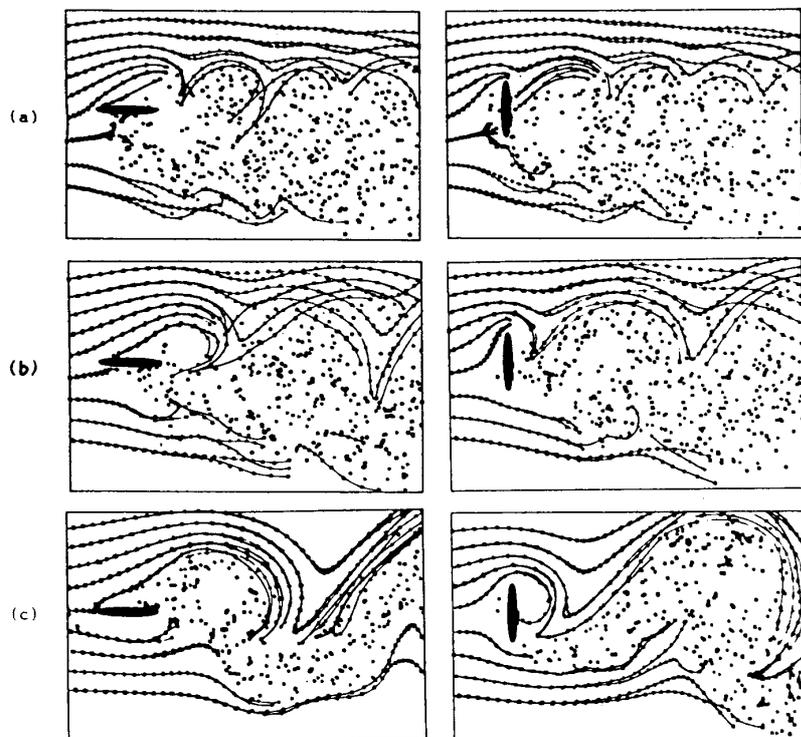
Fig. 6. Numerically simulated streak lines at phase angles of 0 and 90 degrees. The pairs of two from top to bottom correspond to the Strouhal number of 0.4, 0.2 and 0.1, respectively.
