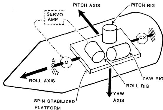
Fig. 3. Attitude measurement unit.
