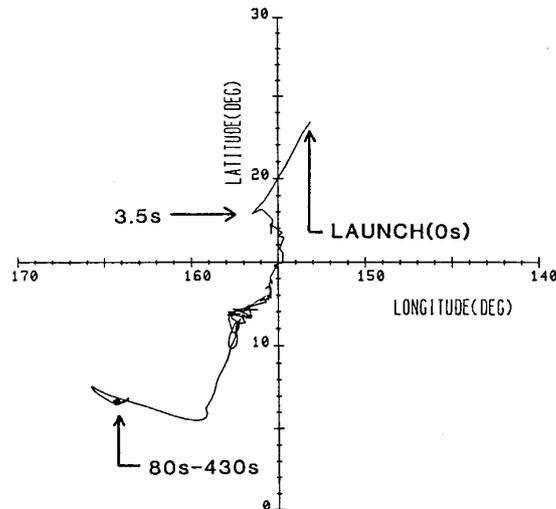
Fig. 7. Locus of nose direction determined by gyro. The nose direction of the rocket is shown. At about 80 s, the initial attitude was acquired which was maintained till 430 s. In the initial 3.5 s period, a sharp nose dive can be observed followed by a precession, nutation and wobbling.
