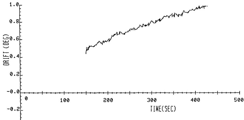
Fig. 8. Gyro drift in longitude direction vs. time. Gyro drift calculated by the sun sensor data is shown. During free flight, a drift of 0.1 deg. per second is observed.
