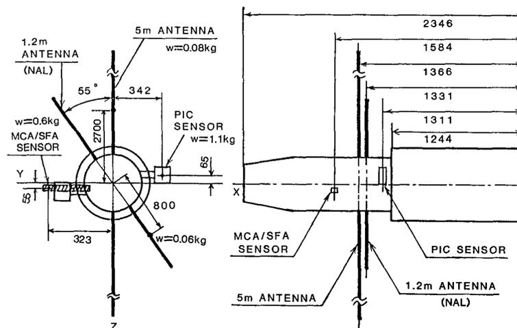
Fig. 1. Deployable antennas and sensors of S-520-5.
