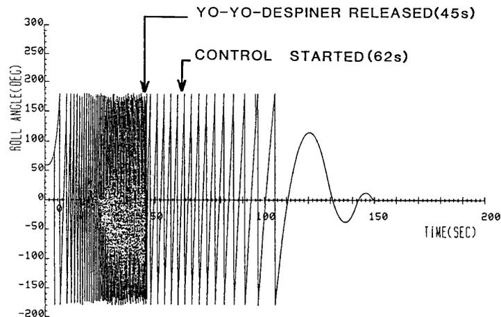
Fig. 6. Roll angle vs. time. Roll angle is shown between  $-180$  deg. and  $+180$  deg. Immediately after the launch, spin was accelerated aerodynamically reaching 2 rps. At 45 s, it was reduced to 0.3 rps by a yo-yo despinner and after 62 s, it was further reduced by side jets.
