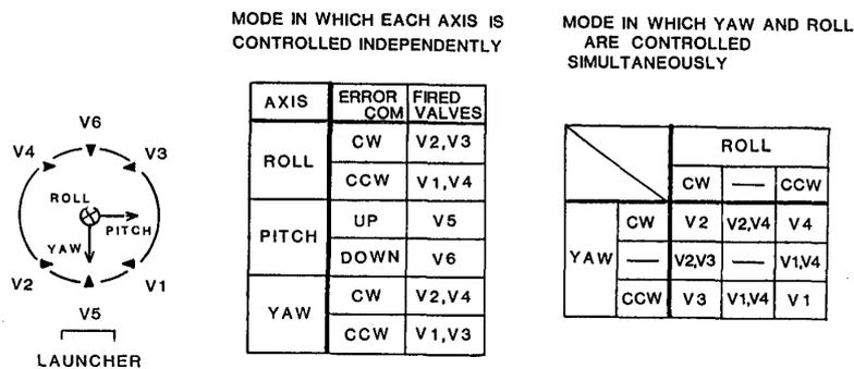
Fig. 2. Engine configuration and its firing logic.
